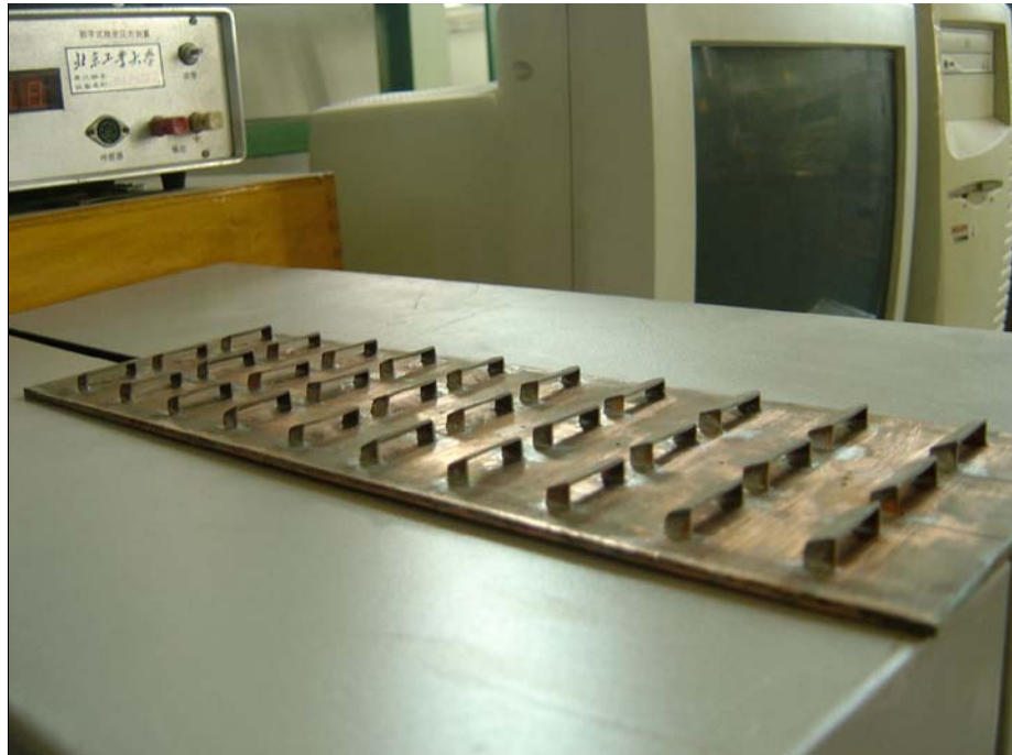
Figure 2. The experimental enhanced duct wall with 3D flow-inclining fins
